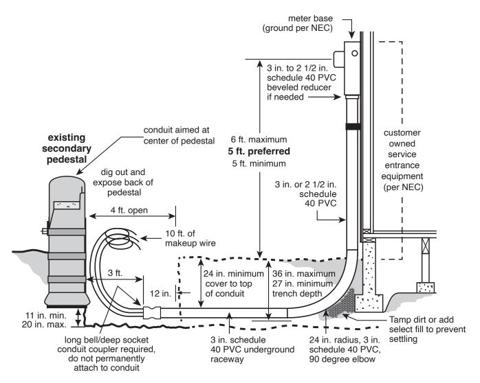
**NOTE:** 3 in. to 2 1/2 in. reducer (if needed) may be installed at the meter base knockout or in the down pipe at the top of the elbow.
