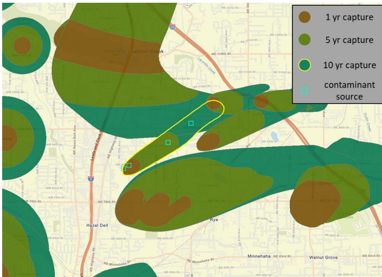
Figure K-6. Map of well #20– 1-, 5-, and 10-year capture zones and the contaminant sources located within them.
