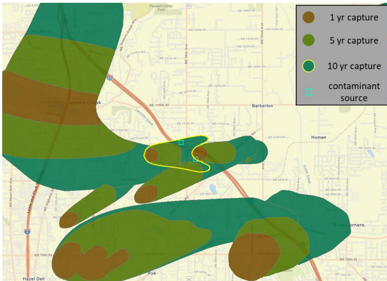
Figure K-7. Map of well #22– 1-, 5-, and 10-year capture zones and the contaminant sources located within them.
