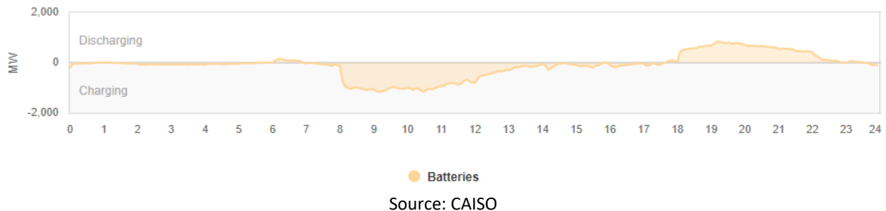
Figure 4.11 CAISO Battery Fleet Hourly Charge/Discharge on 8/18/21
