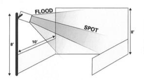
300-WATT FLOOD LIGHT OR SPOT LIGHT MOUNTS ON 8-FOOT UPRIGHT AT FRONT CORNER OF BOOTH.
