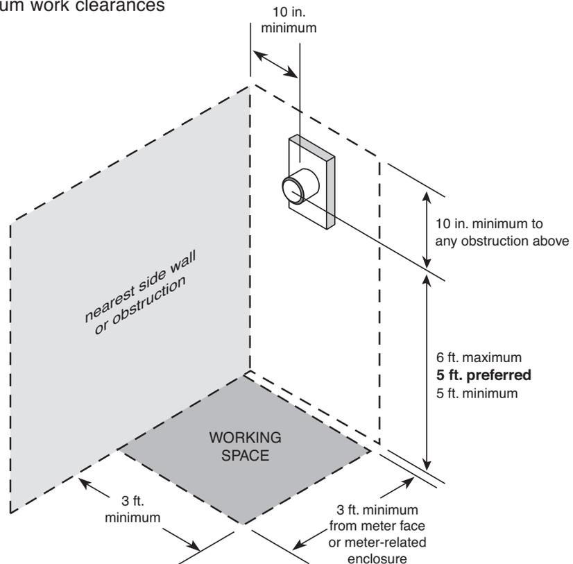
**Figure 20** Recessed meter base detail
