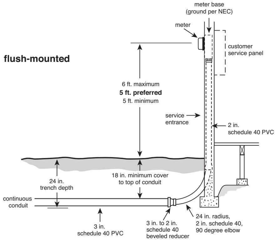
**NOTE:** Flush-mounted service entrance conduit cannot be located in a shear wall or within 4 ft. of a structure corner.
