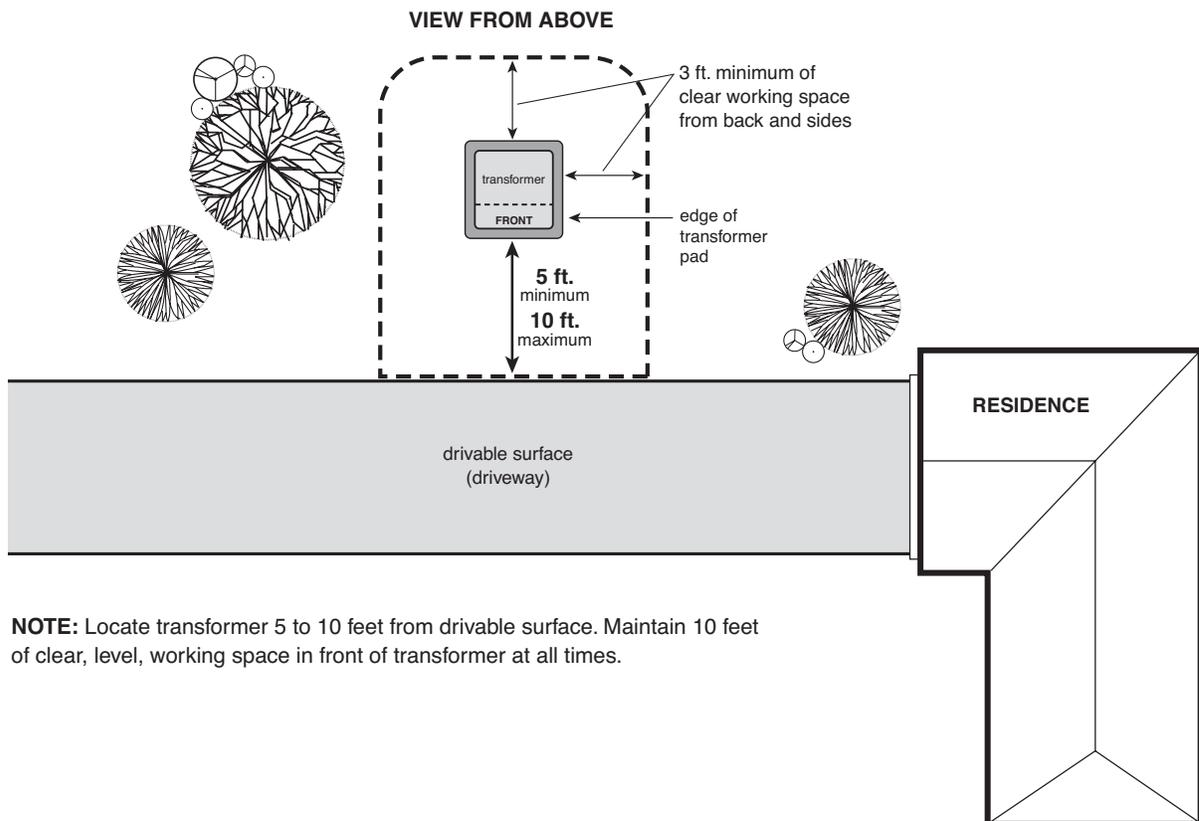
**NOTE:** Locate transformer 5 to 10 feet from drivable surface. Maintain 10 feet of clear, level, working space in front of transformer at all times.
