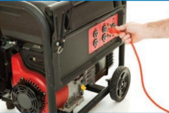
If you use a back-up generator, please do not hook it up or plug it in to your home electric system without first disconnecting from our system. If you don't take precautions, the power from your generator may flow backwards into our power lines and seriously injure or kill our line repair workers.
